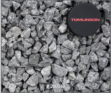
**19mm CONCRETE STONE 3/4"** 5 - 20mm in size. (1/4" - 1")
