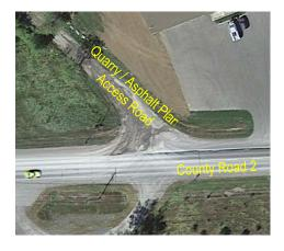
• County Road 2 / Site Access: The proposed asphalt plant would be accessed through the existing access road located approximately 940m east of the County Road 2 / Palace Road intersection. The minor site access is STOP-controlled and is unpaved. It currently provides access to quarry truck traffic.
