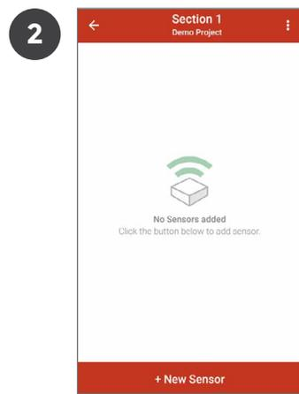
Add a new sensor by pressing + New Sensor.
