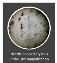
pathways for water and waterborne contaminants. Any moisture introduced over the lifespan of the concrete will initiate crystallization, ensuring permanent waterproofing protection.
